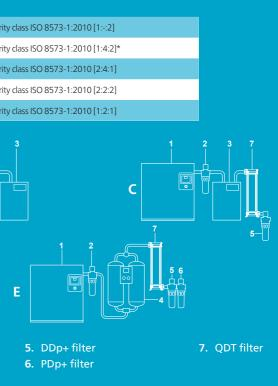
es, it is advised to install particle filters DDp+ and PDp+ just before the applicatior
