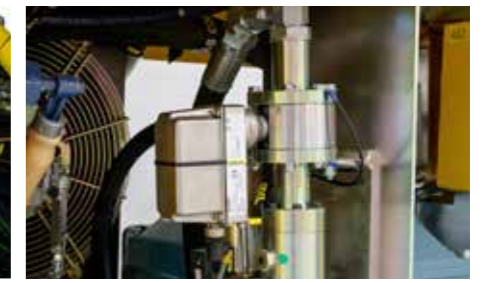
An inductive water flow meter, without moving parts, and a highly accurate pressure sensor increases flushing reliability and availability of the machine.
