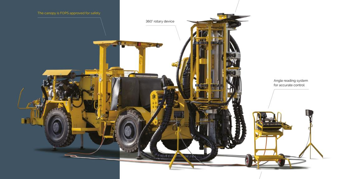
Mobile control panel keeps the operator at a safe distance from the drilling area
