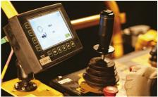
Degitized angle reading system helps operators to fulfill more accurate hole angle and depth.
